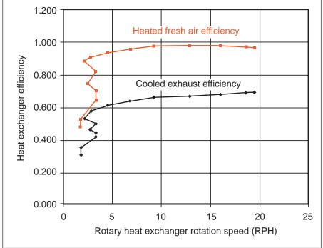
Figure 2: Performance results of the heat wheel at a dryer exhaust temperature of 142 °C.
